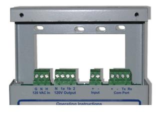
The MC3's durable metal enclosure provides mounting to standard electrical boxes (4"sq., single gang, double gang, handy box etc.) or surface 1/2" conduit entry through 3 top knockouts. Removable wiring cover facilitates easy connections with ample wire cavity. Terminations are to plug-in connectors.
